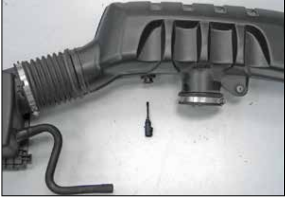
18. Release the locking tab and then remove the inlet air temperature sensor from the factory intake tube by twisting counter clockwise. NOTE: The inlet air temperature sensor is very fragile; take care to avoid damage while handling the sensor.
