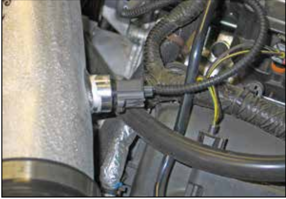
23. Connect the inlet air temperature sensor extension harness into the factory electrical connection and then connect the other end into the inlet air temperature sensor as shown. NOTE: There are two different types of sensors, be sure to choose the correct harness extension for the sensor used.
