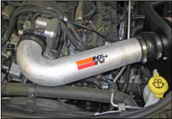
21. Install the K&N® intake tube into the hump hose at the filter adapter and then into the hose at the throttle body. Adjust the tube and heat shield for best fit and clearance and then secure with the provided hose clamps
