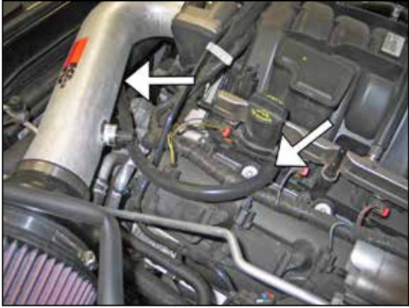
22. Install the crank case vent hose onto the 90° vent fitting and then attach the open end to the valve cover port.
