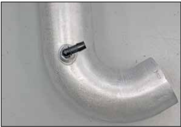
20. Install the 90° npt fitting into the K&N® intake tube as shown. NOTE: Plastic NPT fittings are easy to cross thread. Install the vent fitting “hand” tight, then turn it two complete turns with a wrench.
