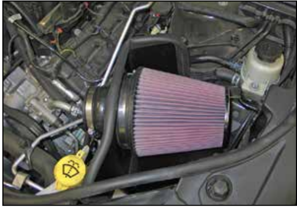
16. Install the K&N® air filter onto the adapter and secure with the provided hose clamp. NOTE: Drycharger® air filter wrap; part # RF-1041DK is available to purchase separately. To learn more about Drycharger® filter wraps or look up color availability please visit http://www.knfilters.com ®.
