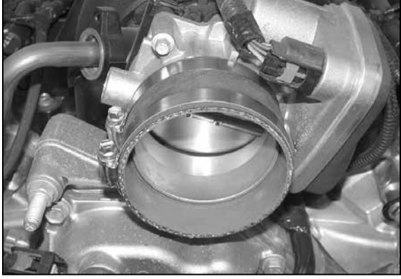
17. Install the provided silicone hose (08630) onto the throttle body and secure with the provided hose clamp.
