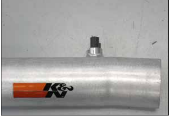
19. Install the inlet air temperature sensor into the K&N® intake tube.
